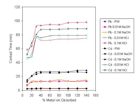
Figure 2. Effect of acidic, basic and neutral media on the recovery of Pb<sup>2+</sup> and Cd<sup>2+</sup> from Caladium bicolor biomass.
