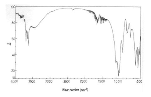
Figure 1. FTIR Spectra of the biomass sample.
