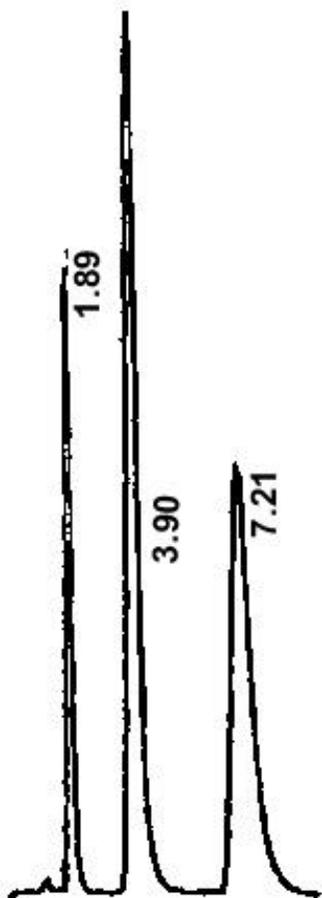
**Figure 2. Representative HPLC chromatogram for flurbiprofen analysis: caffeine (1.89 min), R-flurbiprofen (3.90 min), and S-flurbiprofen (7.21 min).**
