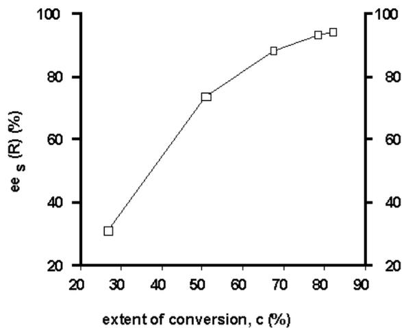
Figure 9. Enantiomeric excess of the R-enantiomer of flurbiprofen as a function of the total substrate converted to product by the *Candida rugosa* lipase-catalyzed reaction in isooctane at 0.65 water activity.
