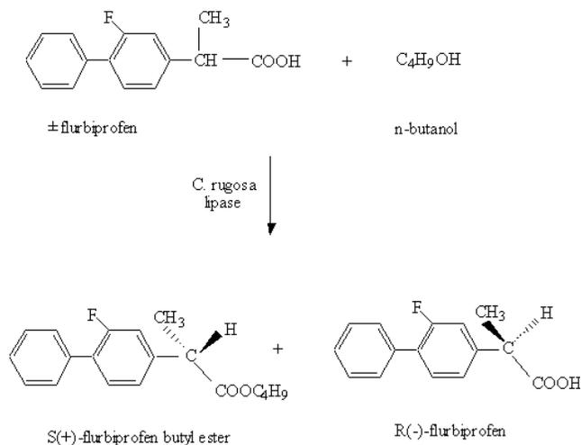
**Figure 1. Reaction scheme for the enantioselective esterification of flurbiprofen with n-butanol.**
