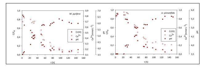
Fig. 2 Cr(III) breakthrough curves for calcium-treated *M. pyrifera* and *U. pinnatifida* biomasses. Empty and closed circle symbols represent calcium release and Cr(III) concentration in the eluate, respectively, while cross symbols indicate pH behaviour during Cr(III) uptake.
