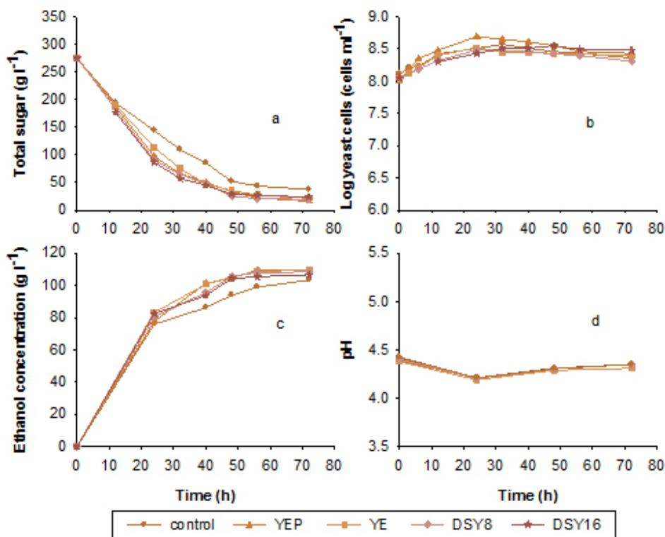
**Fig. 1** Fermentation kinetics during batch ethanol production from the sweet sorghum juice containing 280 g l<sup>-1</sup> of total sugar under various nitrogen supplements by *S. cerevisiae* NP 01. (a) total sugar, (b) log yeast cells, (c) ethanol concentration and (d) pH.
