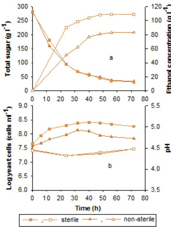
**Fig. 4 Fermentation kinetics during batch ethanol production from sterile and non-sterile sweet sorghum juice supplemented with 8 g l<sup>-1</sup> of DSY by *S. cerevisiae* NP01. (a) total sugar (closed symbol) and ethanol concentration (open symbol), (b) log viable yeast cells (closed symbol) and pH (open symbol).**
