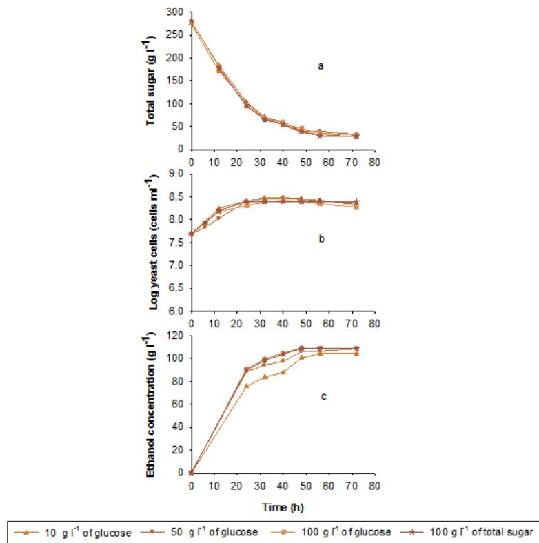
**Fig. 3** Fermentation kinetics during batch ethanol production from the sweet sorghum juice supplemented with  $8 \text{ g l}^{-1}$  of DSY by *S. cerevisiae* NP01 grown in different initial sugar concentrations in IP medium. (a) total sugar, (b) log viable yeast cells and (c) ethanol concentration.
