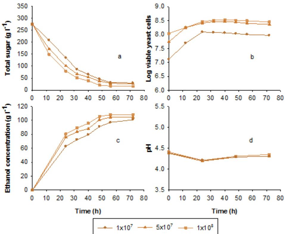
**Fig. 2** Fermentation kinetics during batch ethanol production from the sweet sorghum juice supplemented with  $8 \text{ g l}^{-1}$  of DSY under different initial yeast cell concentrations of *S. cerevisiae* NP 01. (a) total sugar, (b) log viable yeast cells, (c) ethanol concentration and (d) pH.
