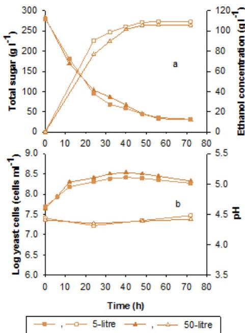
**Fig. 6 Fermentation kinetics during batch ethanol production from the sweet sorghum juice supplemented with 8 g l⁻¹ of DSY in 5-litre and 50-litre bioreactors.** (a) total sugar (closed symbol) and ethanol concentration (open symbol), (b) log viable yeast cells (closed symbol) and pH (open symbol).
