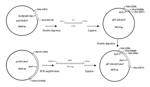
Fig. 1 The procedure of pET-22b-ELP-dhaT construction.
