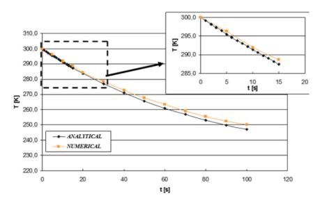
Fig. 3 Comparison of analytical-numerical CFD results.
