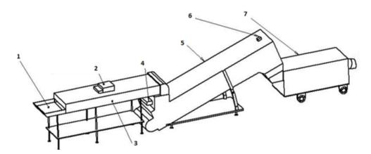
**Fig. 1 Grape rapid cooling machine:** (1) grape inlet hopper; (2) CO<sub>2</sub> injector; (3) vibrating table; (4) CO<sub>2</sub> injector; (5) belt elevator; (6) temperature drill; (7) crusher-destemmer machine.
