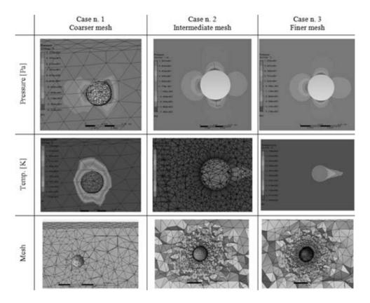
Fig. 2 CFD results for different mesh refinements.
