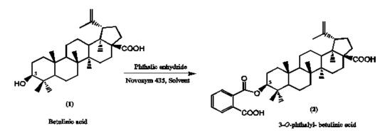
Figure 1. Reaction between betulinic acid and phthalic anhydride using Novozym 435 as biocatalyst.
