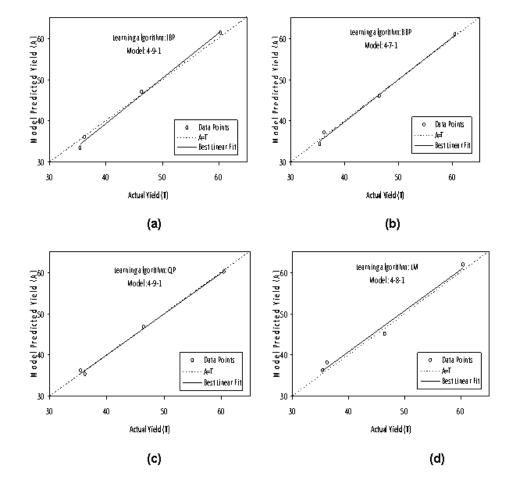
Figure 5. The scatter plots of ANN predicted yield *versus* actual yield for testing data set from: (a) Incremental backpropagation (IBP) algorithm.
