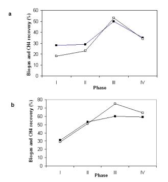
Figure 3. Biogas ( $\blacksquare$ ) and methane ( $\square$ ) recovery for the GCC (a) and the UASB (b) reactors.
