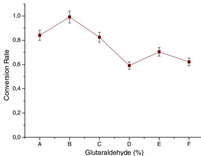
**Fig. 7.** Effect of concentration of glutaraldehyde on the production of D-CpHPG. From 0.0% to 1.0% the fluctuating concentration of glutaraldehyde increased by 0.25%. Reagents and conditions: LB (200 mL), DL-HPH (1.9 g), bead diameter = 2.60 mm, pH = 8.0, T = 37°C, 3.0% sodium alginate, 1.5% diatomite, samples were taken at 48 h. A: free cells; B: 0.0%; C: 0.25%; D: 0.5%; E: 0.75%; F: 1.0%.
