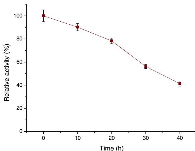
**Fig. 4.** Thermostability of D-hydantoinase. The purified enzyme was tested by incubation, without substrate, for different times (10, 20, 30, 40 h) in 100 mM sodium phosphate buffer pH 8.0 at 40°C. The residual activity was measured, with the original activities of D-hydantoinase, without pre-incubation, being defined as 100%.
