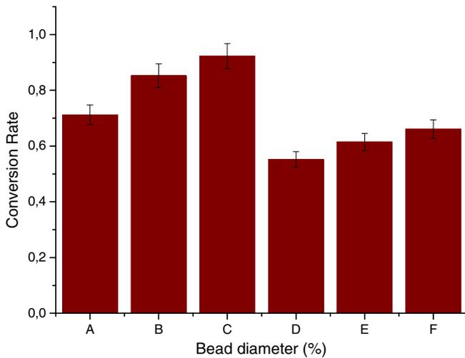
**Fig. 8.** Effect of bead diameter on the production of D-CpHPG. Reagents and conditions: LB (200 mL), DL-HPH (1.9 g), pH = 8.0, T = 37°C, 3.0% sodium alginate, 1.5% diatomite, samples were taken at 48 h. A: free cells; B: 2.27 mm; C: 2.60 mm; D: 3.03 mm; E: 3.54 mm; F: 4.00 mm.
