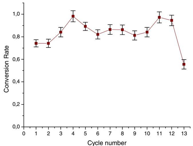
**Fig. 11.** Effect of repeated batch fermentation on the production of D-CpHPG. Reagents and conditions: LB (200 mL), DL-HPH (1.9 g), bead diameter = 2.60 mm, pH = 8.0, T = 37°C, 3.0% sodium alginate, 1.5% diatomite, 0.05%  $CaCl_2$ , 1.0 mM  $MnCl_2$ , samples were taken at 48 h.
