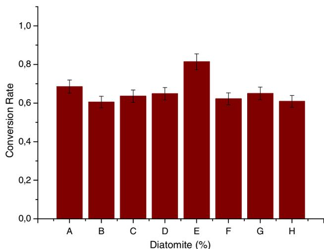
**Fig. 6.** Effect of concentration of diatomite on the production of D-CpHPG. From 0.0% to 3.0% the fluctuating concentration of diatomite increased by 0.5%. Reagents and conditions: LB (200 mL), DL-HPH (1.9 g), bead diameter = 2.60 mm, pH = 8.0, T = 37°C, 3.0% sodium alginate, samples were taken at 48 h. A: free cells; B: 0.0%; C: 0.5%; D: 1.0%; E: 1.5%; F: 2.0%; G: 2.5%; H: 3.0%.
