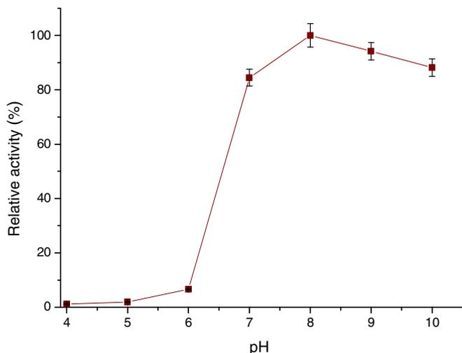
**Fig. 3.** Effects of pH on the specific activity of purified D-hydantoinase. The enzymatic activity was measured at 40°C using 100 mM sodium acetate buffer (pH 4–6), 100 mM sodium phosphate buffer (pH 6–8) and 100 mM sodium carbonate buffer (pH 9–10) with the substrate.
