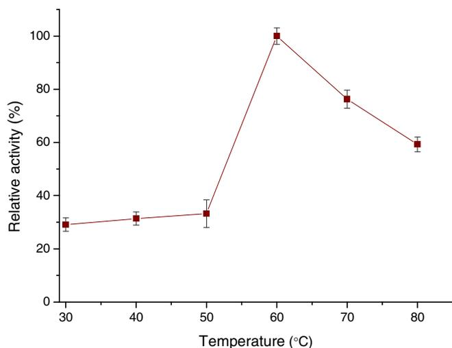
**Fig. 2.** Temperature optimization. The enzymatic activity of D-hydantoinase was measured in sodium phosphate buffer (pH 8.0) for 10 min at 30, 40, 50, 60, 70, and 80°C.
