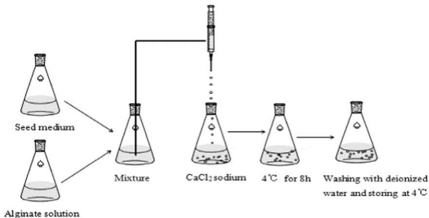
Fig. 1. Flow chart of whole cell immobilization: first, an 18 h seed culture and alginate solution were compared; second, the mixture of seed medium and alginate solution was passed through a syringe into 200 mL CaCl<sub>2</sub> (3%, W/V) solution in bacteria-free environment to produce beads; third, the CaCl<sub>2</sub> solution with beads was stored at 4°C for 8 h; fourth, the beads were washed with deionized water and stored at 4°C.
