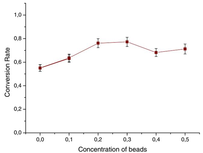
**Fig. 10.** Effect of bead concentration on the maximum production of D-CpHPG. From 0.0% to 50% the fluctuating concentration of beads increased by 10%. Reagents and conditions: LB (200 mL), DL-HPH (1.9 g), bead diameter = 2.60 mm, pH = 8.0, T = 37°C, 3.0% sodium alginate, 1.5% diatomite, 0.05%  $CaCl_2$ , 1.0 mM  $MnCl_2$ , samples were taken at 48 h.
