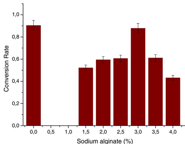
**Fig. 5.** Effect of concentration of calcium alginate on the production of D-CpHPG. From 0.0% to 4.0% the fluctuating concentration of sodium alginate increased by 0.5%. Reagents and conditions: LB (200 mL), DL-HPH (1.9 g), bead diameter = 2.60 mm, pH = 8.0, T = 37°C, samples were taken at 48 h.
