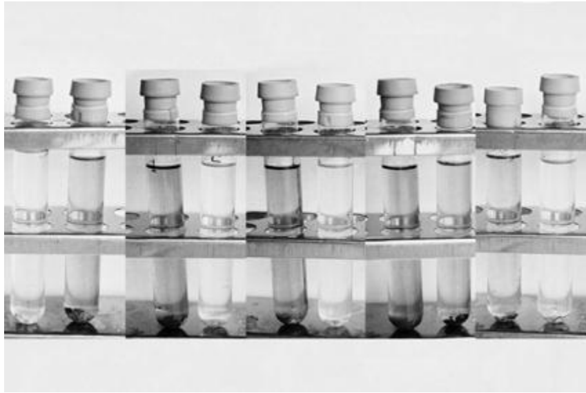
Figure 7. View of melted teeth block specimens in 50% Nitric acid solution.
